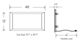
Flush Mount must be installed on a hard ceiling.
